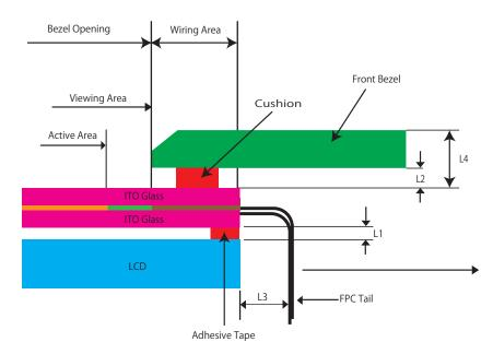
L4≧2mm: Distance between touch screen and bezel surface
