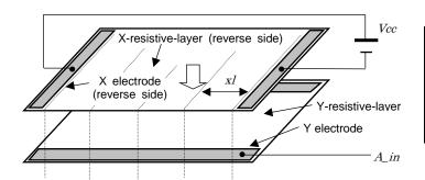
Vcc = 5.0VχĮ A\_in **Output Data** Α 0V 0000h (Min.) В 1.25V 00FFh С 2.5V 01FFh 02FFh D 3.75V Ε 5V 03FFh (Max.)
