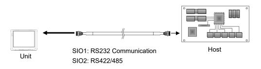
\*Applying Ferrite Core to the communication cable is recommended for noise and static measures.
