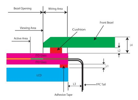
L4≧2mm: Distance between touch screen and bezel surface
