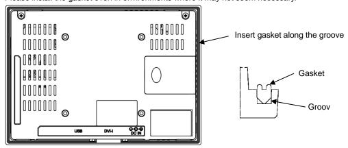
XGasket will be installed to the unit before shipment.
