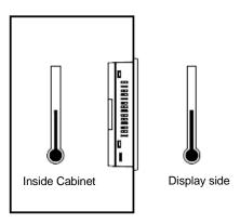
• TM should be mounted perpendicular, but if it should be mounted in an angle, the angle shall not be more than 30degrees from the vertical position shown in the illustration below.
