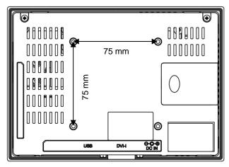
Use M4 screws to mount. The tightening torque range is 0.7~0.8N ⋅ m.
