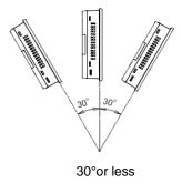
• When installing the TM in a slanted panel of angle 30 degrees or more, please use forced air cooling to ensure the temperature specification.
