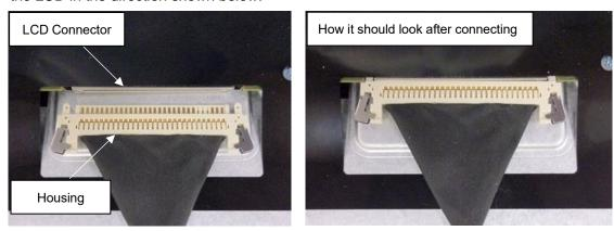
(2) Slide and connect the housing of the image cable to the Power connector on the back side of the LCD as shown in below diagram.
